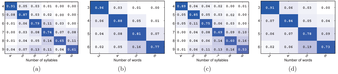
Figure 9: Automatic segmentation accuracy for (a) inner-word segmentation on commercial devices; (b) inter-word segmentation on commercial devices; (c) inner-word segmentation on USRP; (d) inter-word segmentation on USRP.
